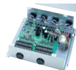
CZ-CAPDC Serial parallel device controlling outdoor units, up to 4 units.
